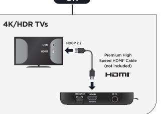
To stream 4K or HDR. choose an HDMI port that supports **HDCP 2.2**. Use a Premium High Speed HDMI® Cable (not included).
